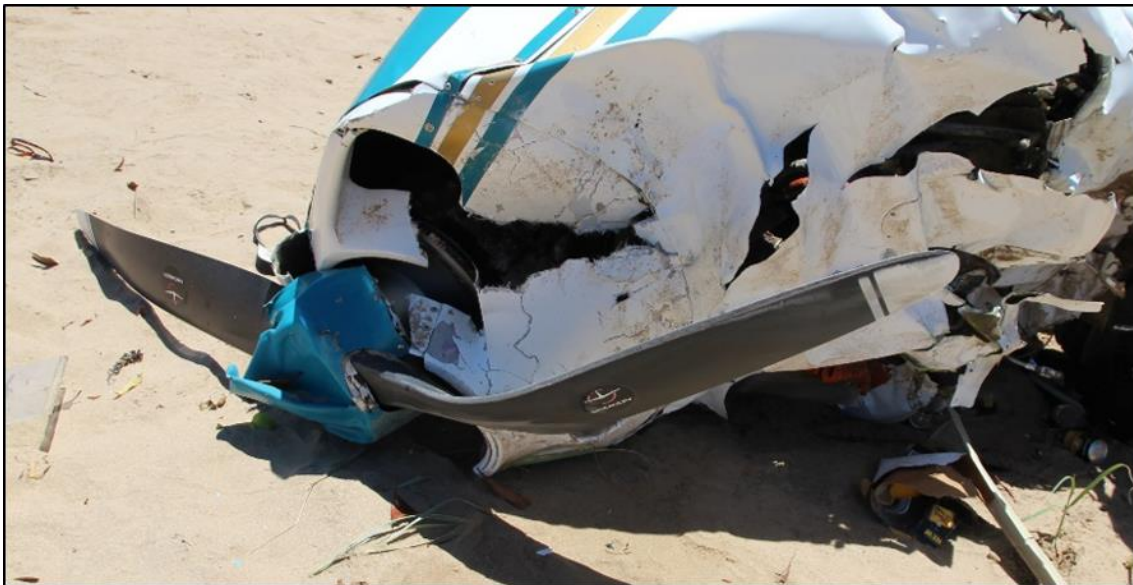
Figure 14: Propeller blades showing slight paint abrasion damage
