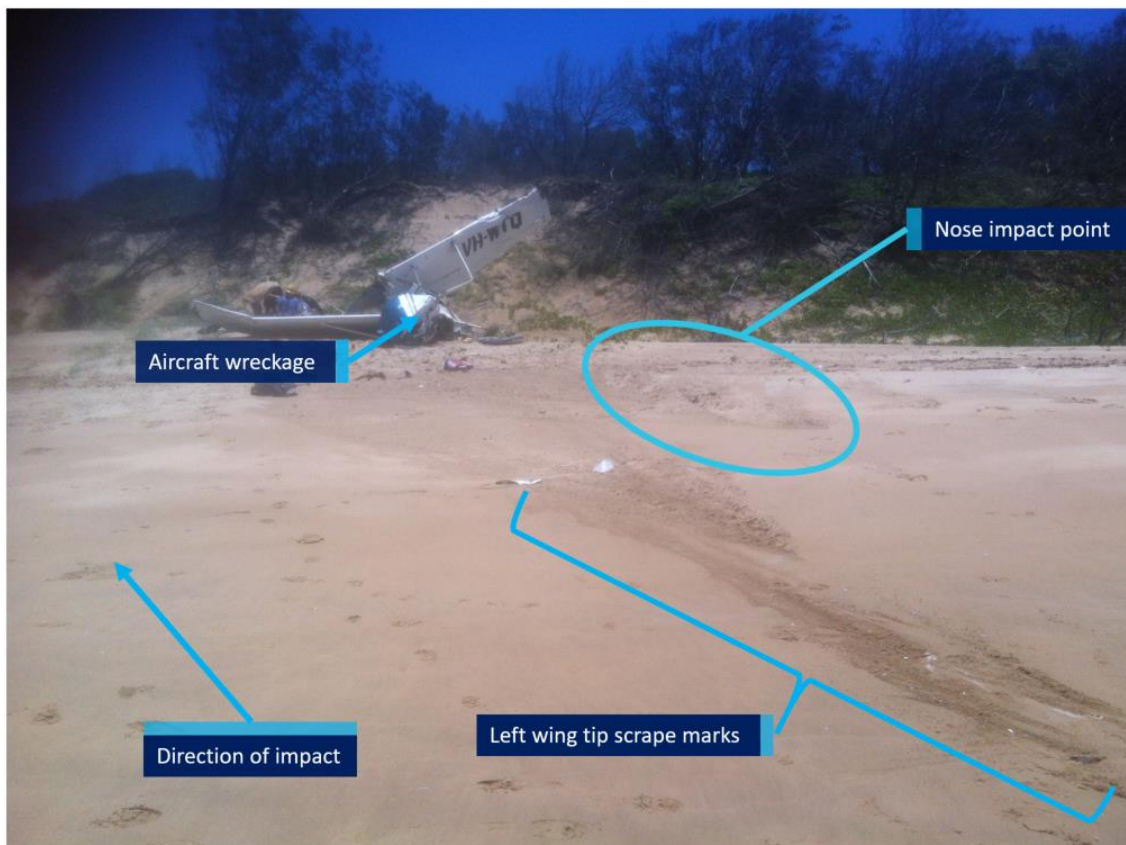
Figure 8: VH-WTQ accident site showing impact marks
