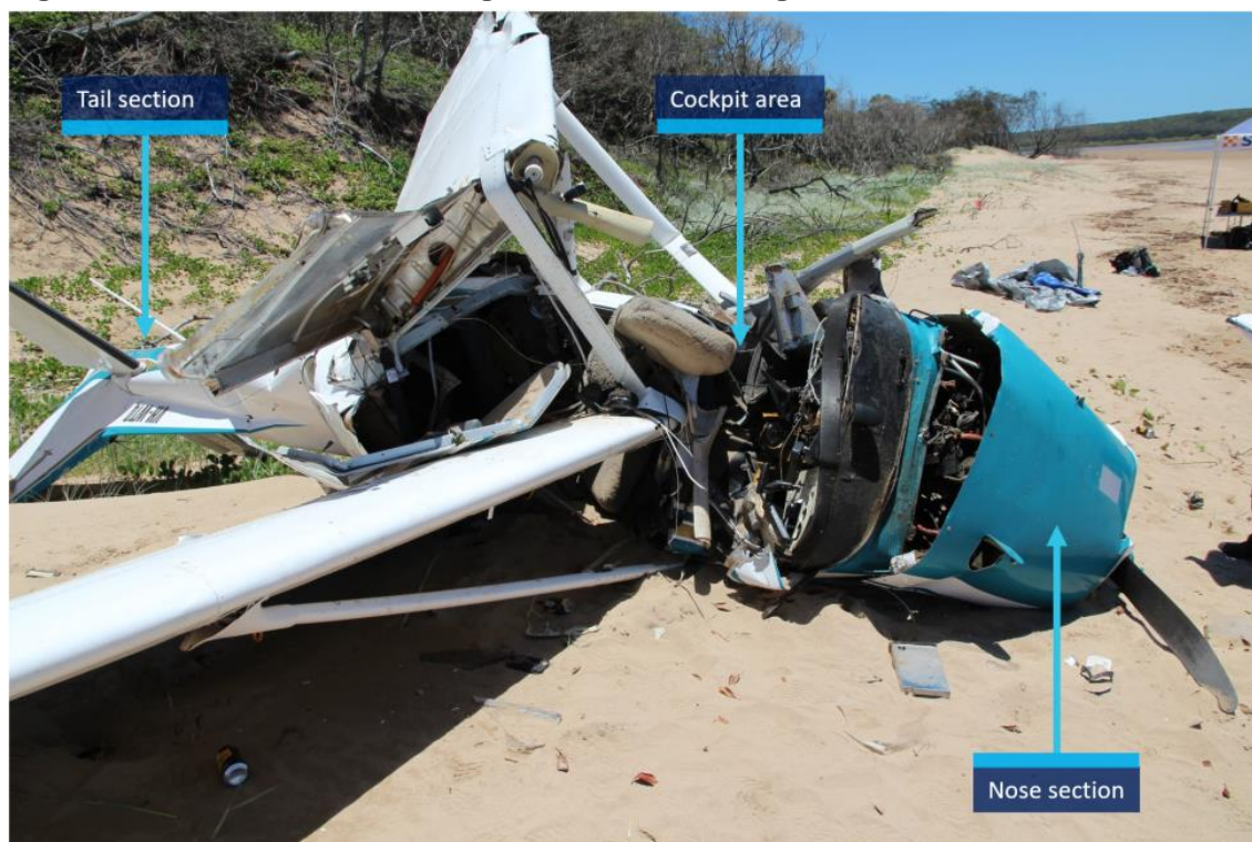
Figure 9: VH-WTQ aircraft wreckage viewed from the right
