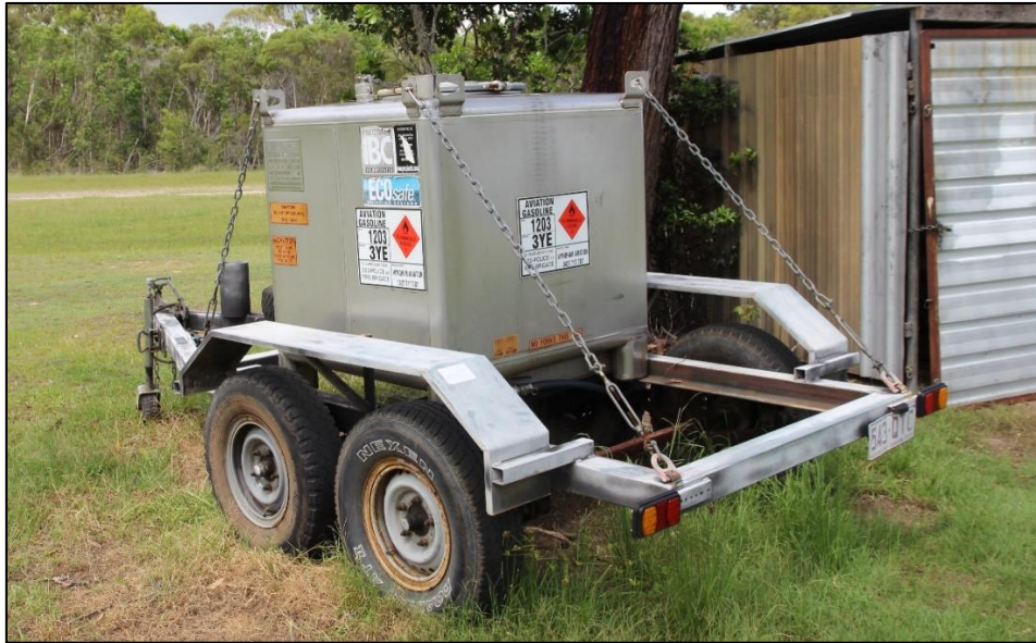
Figure 15: Fuel storage tank containing aviation grade gasoline
